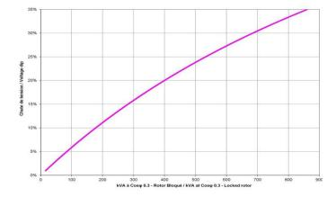
Peak motor starting (kVA) based on x% voltage dip power factor at 0.3
